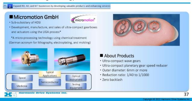
Next, please refer to page 37. The products on a finger in the picture are made by a subsidiary of the German subsidiary, a sub-subsidiary, using the LIGA process. It isn't made by cutting, but made by chemical processing. This is also used in the very minute driving parts of inspection devices for semiconductors.
